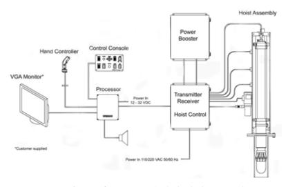
System Components include: dash mounted console and hand-held controller.
