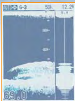
Single freq (50 kHz) with A-scope, Reverse mode
