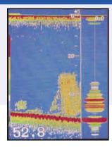
The A-Scope picture on the right 1/3 of the screen shows an instantaneous echo envelope at each ping, clearly showing echo differentials and positional relationship. This is useful for closer observation of target depth.
