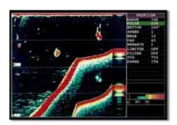
Full Screen Sounder for rough days when conventional sounders lose picture, the sonar transducer can be locked down for a reliable stabilized sounder picture with zoom. White line is available to distinguish fish from bottom.
